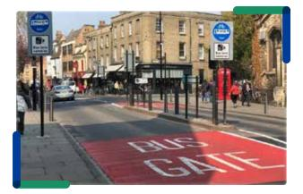
A Bus Gate is a sign-posted short length of stand-alone bus lane. This short length of road is restricted exclusively to buses, taxis and cyclists plus emergency vehicles. It facilitates bus priority by removing general through traffic along the overall road where the bus gate is located. General traffic will be directed by signage to divert away to other roads before they arrive at the Bus Gate.
